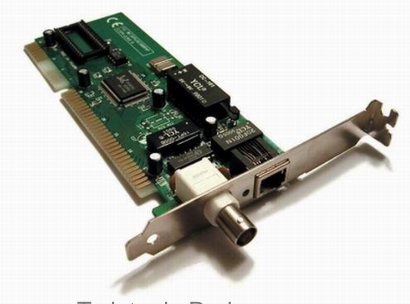
Tarjeta de Red con conector BNC (cable coaxial) y conector RJ45
